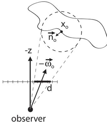
Figure 2: The filter kernel, of size  $d$ , is determined per pixel by a projection of the bounding sphere of radius  $r_{max}$ .
