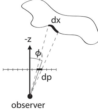
Figure 1: In this figure the relation between the differentials  $dx$  and  $dp$  is illustrated.
